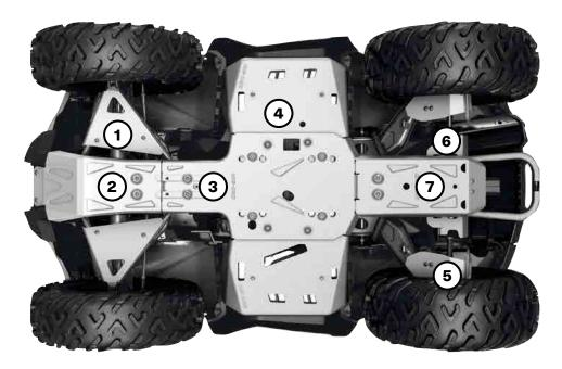
For ultimate durability and strength, all our Aluminum Skid Plates are made with ¾6" (4.5 mm) thick High Strength 5052 H32 Aluminum.
